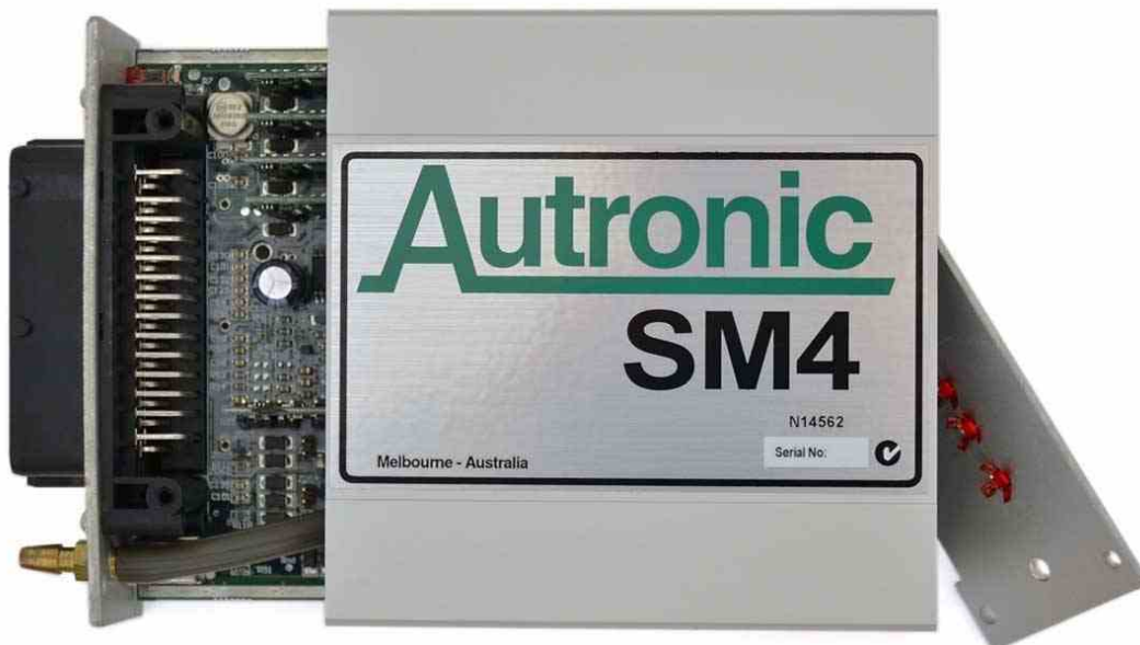
Figure 8 Slide Rear End plate & PBC into SM4 case (same as SM3)
